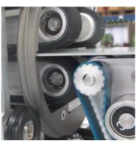
The tilting module is designed to rotate parts such as wafers or displays. The parts are «turned upside down», i.e. rotated around the transport axis. The parts are loaded onto and discharged from the tilting module by means of belt conveyors. The tilting module features special belts of foamed material, which are very soft and firmly press the parts without damaging them. This concept ensures a delicate and harmless handling of all parts.
