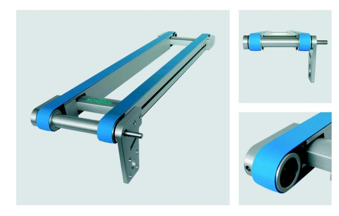
The Special Conveyors SOLTB are used as feed or removal conveyors or for interlinking entire production lines; they are available with flat belts or as a special version with toothed belts. The Special Conveyor consists of a chassis with two belts which are guaranteed to run synchronously. The complete conveyor can be installed and removed from above, and belts can be replaced while the conveyor is installed.
