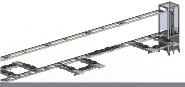
Vertical Lift connection for retraction of workpiece carrier
