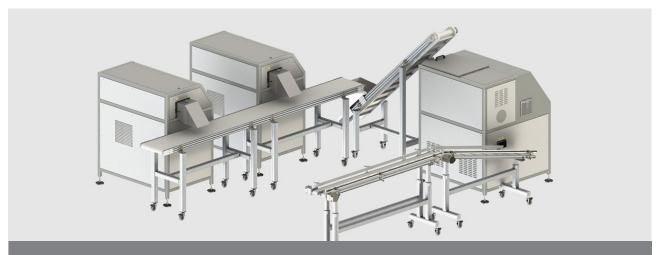
Automation in dry ice production Conveyor System
