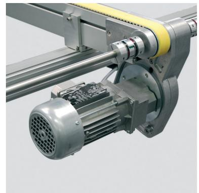
To convey large-scale and heavy work pieces, Montech offers a multitrack conveyor with belts or toothed belts, which can carry weights up to 120 kg. The conveyor is available with three different drives with spur gear motor.
